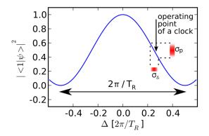
The central frequency-domain Ramsey fringe. Clocks are operated at the point of highest slope, where the transisition probability is the most sensitive to  $\delta$ . Here, a given error  $\sigma_p$  on the measurement of the transition probability translates into a minimal error  $\sigma_{\delta}$  on the frequency measurement.
