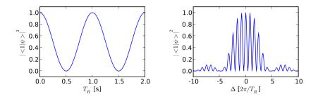
Ramsey fringes in the time domain (left, for  $\delta = 2\pi \times 1$  Hz) and the frequency domain (right).
