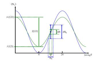
Illustration of projection noise reduction on a Ramsey interference signal.
