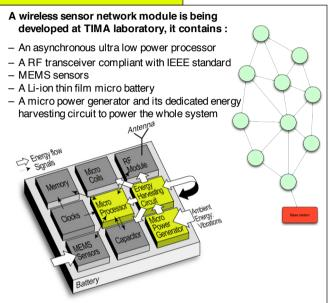
One of the main problems for these microsystems is the power source. For the moment, most of them use a non rechargeable battery, characterised by a finite amount of stored energy, an important volume and mass that dominates the entire system.
