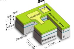
Ambient vibrations induce movement of the mass, and therefore deformation of the cantilever. The compression - elongation (first mode) of the piezoelectric layer creates electric charges that are collected by the electrodes (Silicon beam and Al layer) and transferred to the load. The latter must be tailored to maximise the power transfer
